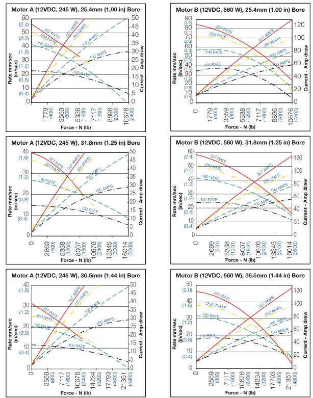
Current draw for Motor C (24VDC, 245 W) and Motor D (24VDC, 560 W) will be approximately ½ of Amp draw shown above.
